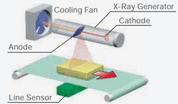
X-rays irradiate items to be inspected that are traveling on the conveyor. A proprietary 5-level image analysis technique is applied to the x-rays that pass through the object and are received by the line sensor, making it possible to detect and eject mixed-in foreign objects, defects, etc.
