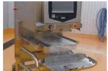
An optional non-contact interlock switch for the protective curtain simplifies attachment and removal from the main body, reducing the risk of damage to the switch.
