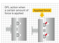
ISHIDA's proprietary Dislocation Force Limiter dissipates the impact when external loads exceed a maximum threshold, preventing damage to weighing sensors.
