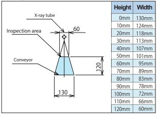
The figures above show the permissible inspection range. Portions of the product which are not within the shaded area are not irradiated.
