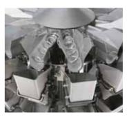
With the arrival of the screw feeder weigher, it is at last possible to apply the recognised, reliable accuracy of Ishida multihead weighing to even the stickiest fresh poultry and meat.
