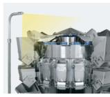
A camera installed in the discharge chute enables constant monitoring of product condition or deposits on the HMI and guides operators to optimize timing setting. Operators can check and adjust production status on the HMI screen.
