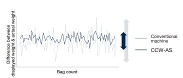
Minimum differences between displayed and actual weight with high weighing accuracy
