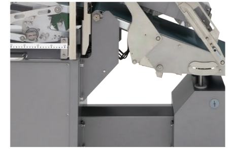
Sloping design prevents dust build up.
