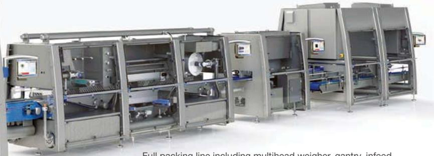
Full packing line including multihead weigher, gantry, infeed, conveyor, batching table, traysealer, X-ray inspection, seal testing, labelling, vision system and pick-and-place case packing.
