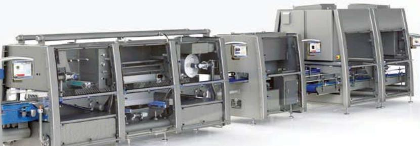
Full packing line including multihead weigher, gantry, infeed, conveyor, batching table, traysealer, X-ray inspection, seal testing, labelling, vision system and pick-and-place case packing.
