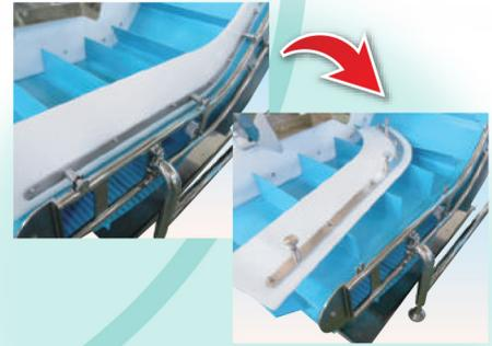
Food grade resin guide provides less friction in between the belt and guide to extend the belt life.
