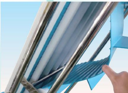
Pipe frame construction provides more accessibility for easy sanitation.
