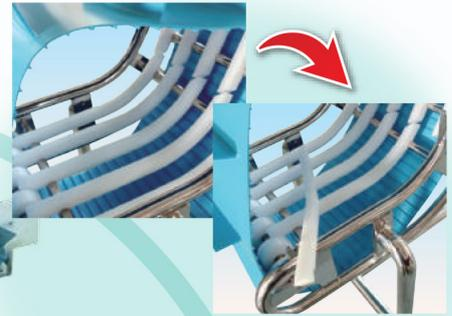
Food grade resin belt carrier rails are light and durable. No tools are required for sanitation and maintenance.
