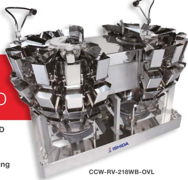
enable high speed weighing up to 280 weigh per minute. With this technology, one oval shape weigher does the job of two weighers, which is big space and cost savings for customers. These technologies are patented in Japan, and now more than 350 units are installed in packaging lines for snacks, biscuits and vegetables factories around the world.
