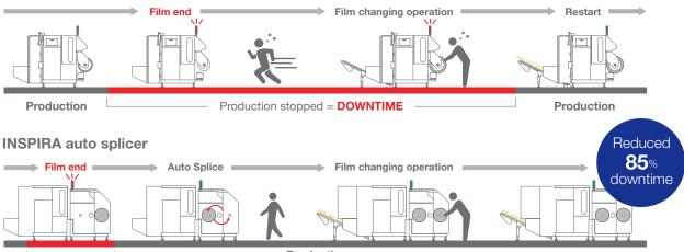
DOWNTIME due to machine stop for Automatic Film Splicing
