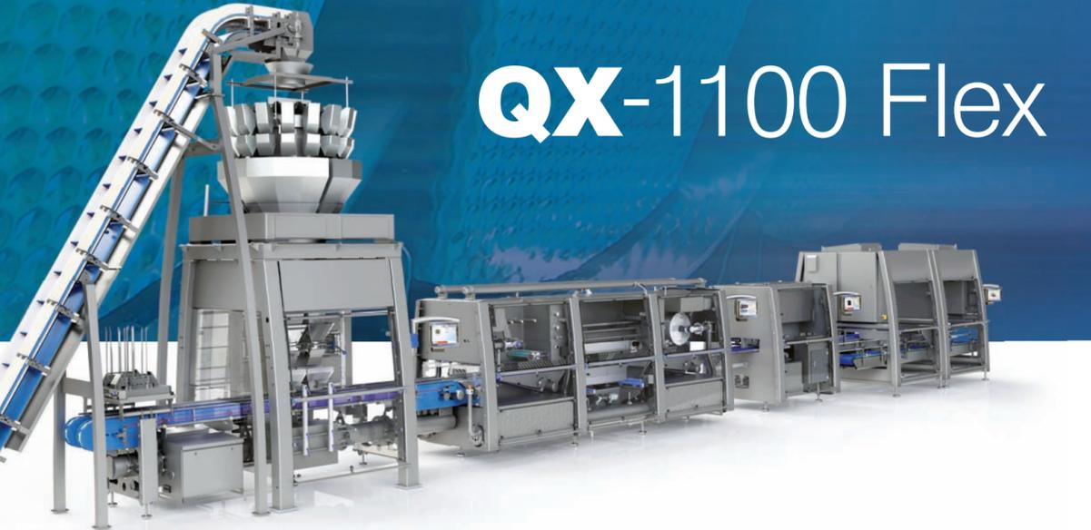
Ishida Europe has launched the new generation of its market-leading QX-1100 tray sealer combined with a brand new concept for the market. The new range offers both single lane and high capacity twin lane models along with the new split dual lane machine which has the capability to operate two independent lanes at different speeds, enabling companies to run two separate tray sizes, pack weights or products at the same time in one machine footprint.
