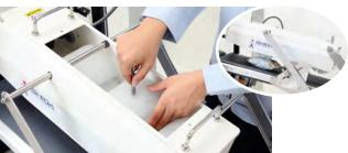
Cleaning brushes under the infeed and inspection conveyors remove product particles and
