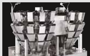
Unique 'two-in-one' Ishida RV-218 multihead weigher over twin rotary-motion Atlas bagmakers
