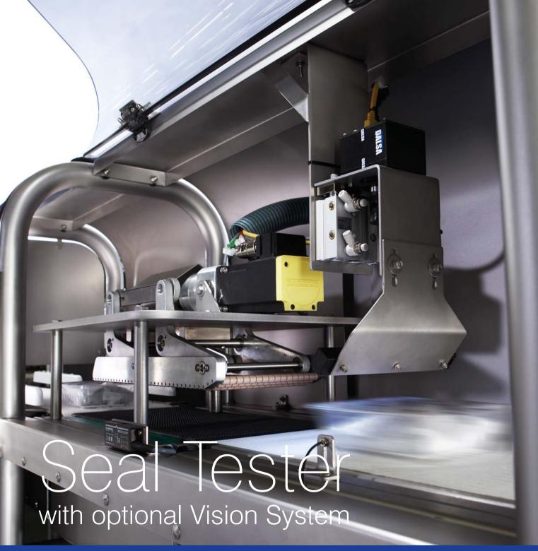
In-line checking of tray and label integrity
