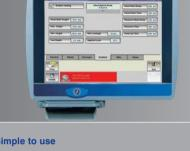
Operators benefit from an easy-to-read touchscreen, with seven languages available. All parameters for each pack type are stored as presets. No cranking of the pressure plate to suit each different tray height: everything adjusts at the touch of a button.
