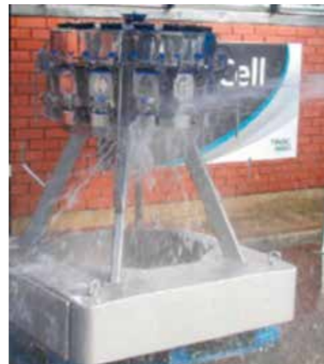
Under-going powerful water jet test for IPX6
