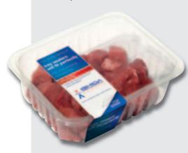
To preserve its attractive colour, the top surface of the meat needs to be exposed to the oxygen-rich modified atmosphere inside the pack. This would be impossible if it were pressed against the top gas-barrier film. So an inner layer of gas-permeable film is included, with a space between the two layers via which the correct atmosphere can reach the top of the meat.
