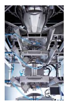
Triple iris design – this allows for the careful orientation and settling of sticks into a compact bundle to achieve the high speed and consistent system performance.
