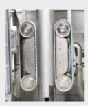
Servomotor control ensure stable feeding of film for reliable packaging at 90 bags/minute.
