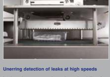
Leak-testing accuracy depends on the ability of the test plate to make smooth contact with the moving tray and apply the correct pressure for long enough to produce satisfactory readings. To achieve this, Ishida uses its own vibration-free servomotor technology and extensive seal-testing experience. The table shows the results.
