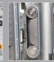
Servomotor control ensure stable feeding of film for reliable packaging at 90 bags/minute.
