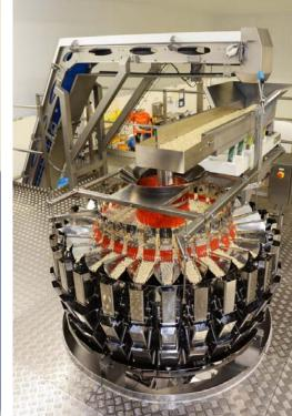
Product giveaway is a cardinal sin and this is something we particularly wanted to address with this new installation. With the Ishida solution, we are now constantly to within a tiny fraction of the target weight.
