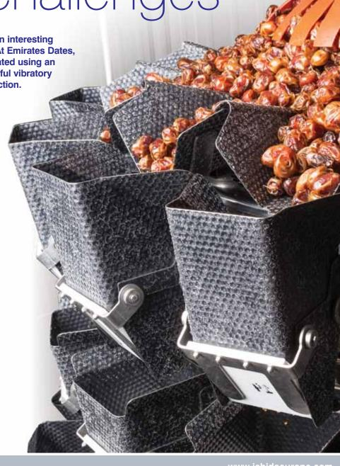
in which powerful spiral screws provide enough propulsion to keep even sticky fresh meat moving. Tests using Emirates Dates products soon convinced the Ishida team that a circular multihead weigher with a really effective vibratory system on board could handle all the challenges.
