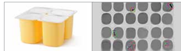
Contamination detection in yogurt pots.
