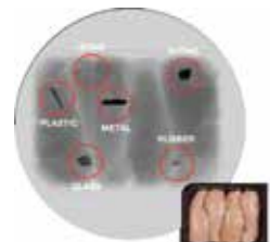
Contaminant detection in chicken
