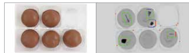
Contamination and missed item detection in chocolate cakes.
